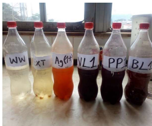
Figure 7. Appearance of wastewater upon addition of green-synthesized nanoparticles; WW : Raw wastewater, EXT : Wastewater + Extract, Ag(1+) : Wastewater + AgNO_3 , VL1 , PP1 , BL1 : Wastewater + Silver nanoparticles
