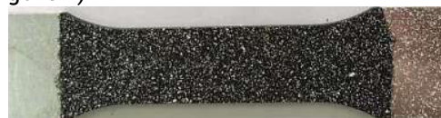
Figure 2. Dog-bone specimen prepared for simultaneous tensile strength – DIC – thermography testing
