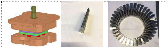
Figure 3. Die press, a single punch, and a set of 36 punches
