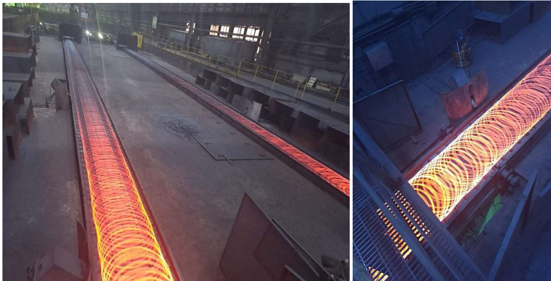
Figure 2. Air Cooling process at STELMOR
