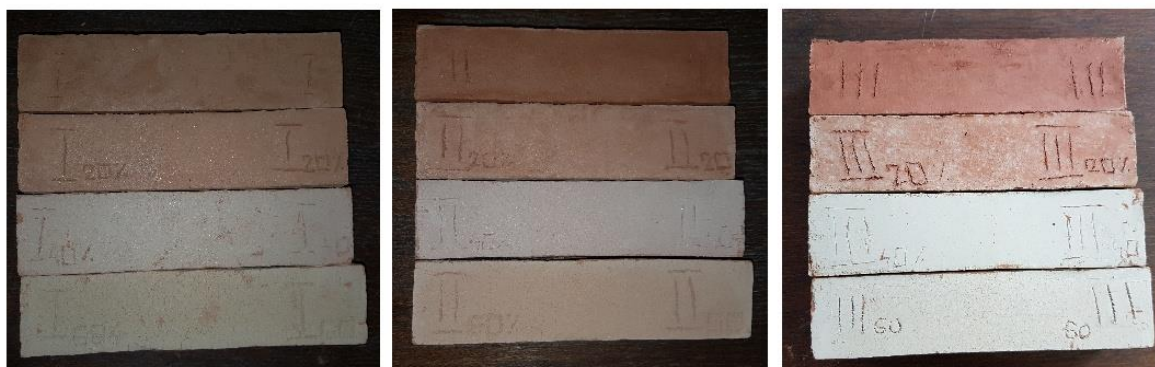
Figure 9. The appearance of prisms after firing (left – firing at 800 °C, middle – firing at 900 °C, right – firing at 1000 °C)
