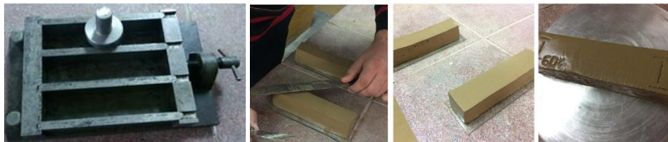
Figure 1. Metal mold for prisms (left) and making and marking prisms (right)
