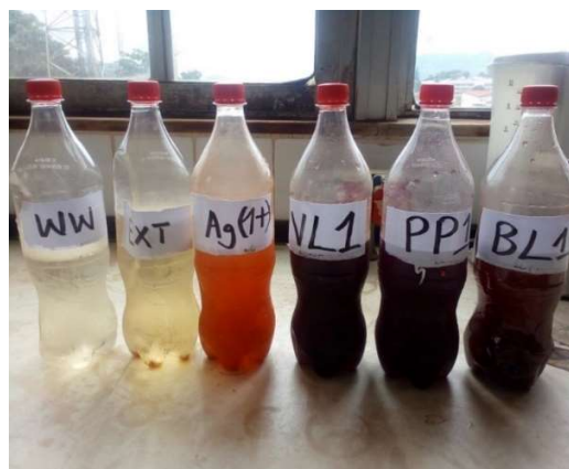
Figure 7. Appearance of wastewater upon addition of green-synthesized nanoparticles; WW: Raw wastewater, EXT: Wastewater + Extract, AG(1+): Wastewater + \text{AgNO}_3 , VL1, PP1, BL1: Wastewater + Silver nanoparticles
