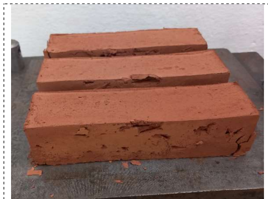
Figure 1. Finished samples of the building block
