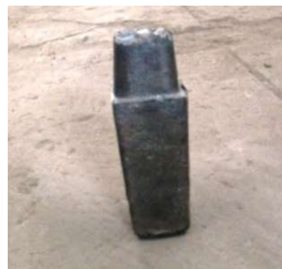
Figure 3. Ingot after the solidification process [7]
