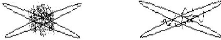
Figure 1. Representation of wet strength mechanism of action: a) protection mechanism, b) amplification mechanism [3]
