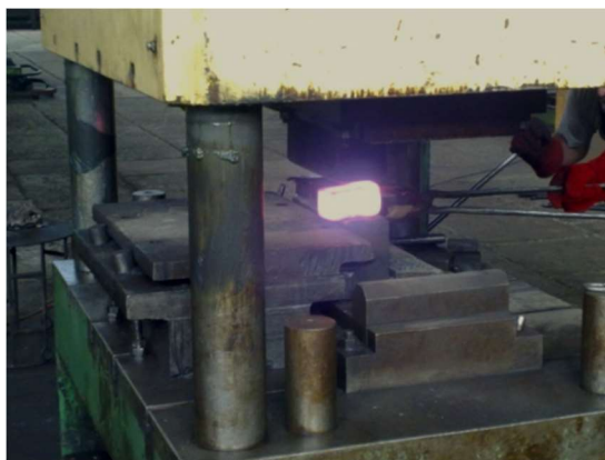
Figure 1. Forging of ingots on a hydraulic press
