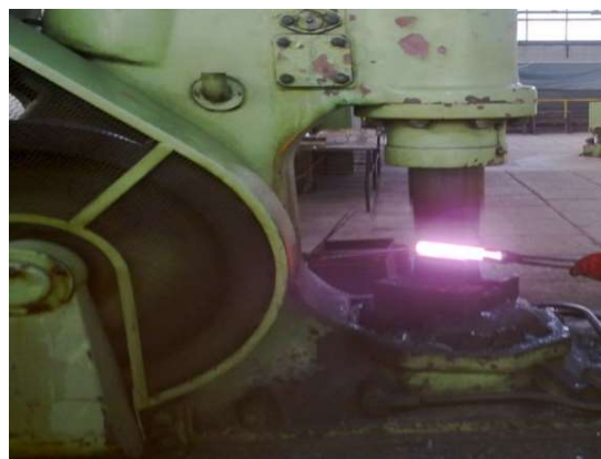
Figure 2. Forging ingots on an air hammer
