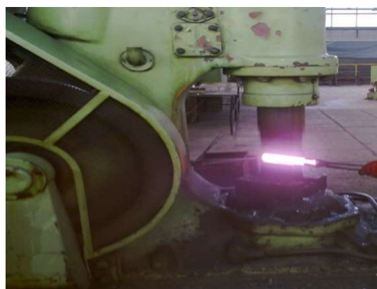
Figure 2. Forging ingots on an air hammer
