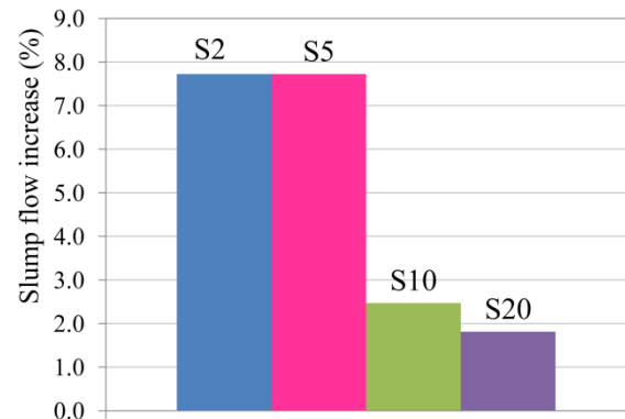
Figure 2. Slump-flow variation of SPC with sulfur compared to the reference sample
