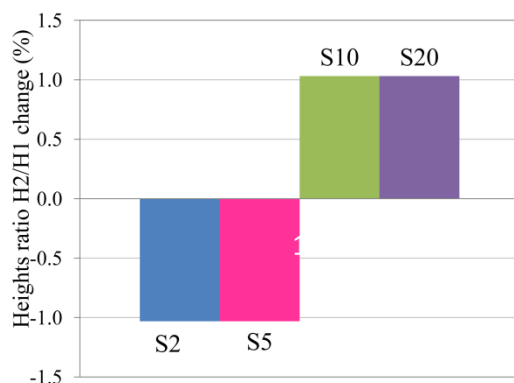
Figure 4. Heights ratio ( H_2/H_1 ) variation of SPC with sulfur compared to the reference sample
